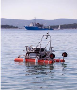
Length 2,00 m Beam 1,10 m Weight 120 kg Draft 0,30 m Payload 60 kg Propulsion Electric Communication range **GSM** network Speed, max 2 km/h Range 6 km
