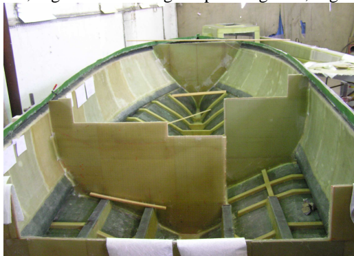
Fig. 12. Production of the prototype hull
