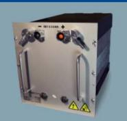
A lithium battery of 100 volts and 6.5 kWh. The connection of + and – are placed on the two inner connectors, and the two outer connectors are for the water cooling.
